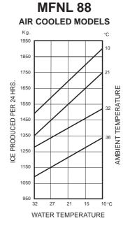
NOTE. Daily ice capacity is directly related to condenser air and water inlet temperature, water temperature to make ice - and age of machine.
