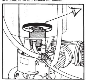
NOTE. The MF/MFN 88 is equipped with a 3 Phase Monitoring Relay (F1). In case the three phase are connected in wrong way, the machine doesn't start with the simultaneous glowing of the 3 Phase Sequence Protector Warning light. Just reverse two of the three phases on the main plug so to have the correct sequence and by so, the start up of the machine.
