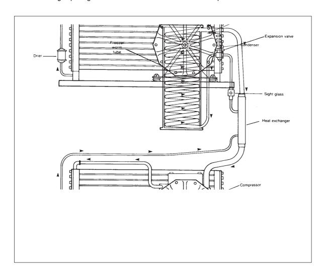
As it evaporates, it absorbs heat from the evaporator and whatever is in contact with it (such as the water inside it). After the evaporator, the refrigerant, now a low pressure vapor, goes through the heat exchanger and suction line back to compressor, where the cycle is repeated.
